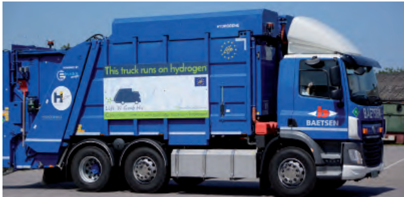
WaterstofNet in Turnhout, Belgium, fuel zero-emission bin lorries with hydrogen.
